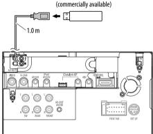
\* Use CA-U1EX to extend the cable if necessary. (Max 500 mA, 5V)
