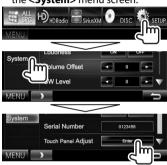
**2** Touch the center of the marks at the lower left and at the upper right as instructed.
