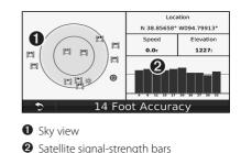
The sky view shows the satellites you are receiving. The satellite signal-strength bars indicate the strength of each satellite you are receiving. A solid bar indicates that the GPS satellite is ready for use.
