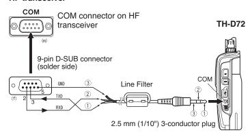
Attach the line filter to the cable.
