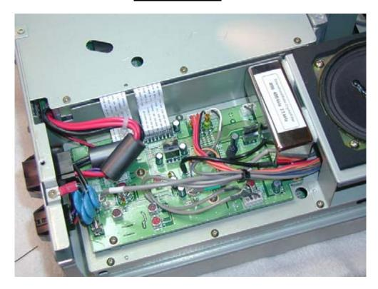
The INRAD #96 filter connects to the Connection Board that is located on the radio top, just behind the speaker.
