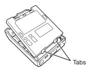
4 To install the battery case onto (or remove it from) the transceiver, follow steps 1 to 3 of "INSTALLING THE Li-ion BATTERY PACK" {above}.
