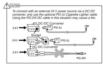
**Note:** If the input voltage exceeds approximately 16.5 V, warning beeps sound and "VOLTAGE ERROR" appears.
