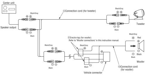
$\ensuremath{\%}$  The high path filter for a tweeter is built in the main part of a tweeter.
