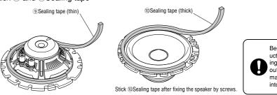
Be sure to install product using provided sealing tape. Installing without using sealing tape may cause water leak into a vehicle
