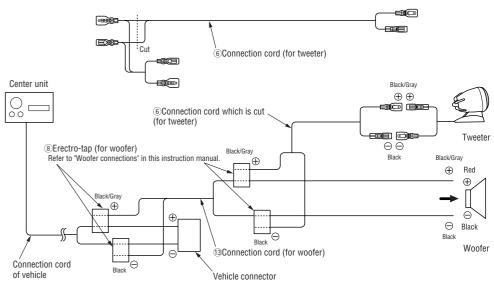
\* The high path filter for a tweeter is built in the main part of a tweeter.
