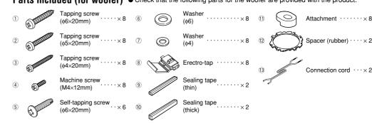
Installation preparation \* Stick 9 and @Sealing tape, in order to prevent vibration and leak.
