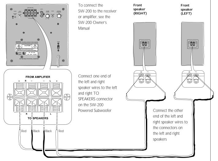
Caution: When connecting the speakers to the amplifier or subwoofer, be sure to always connect the positive ('+') terminals to each other, and the negative ('-') terminals to each other. Connecting the wrong terminals together could damage the amplifier or cause poor sound quality.
