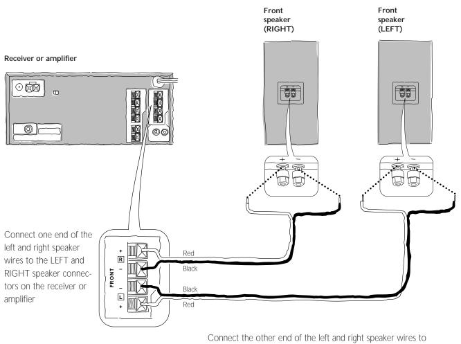
Connect the other end of the left and right speaker wires to the connectors on the left and right speakers. Make sure to connect the positive (+ or red) speaker terminal to the positive terminal on the receiver or amplifier.
