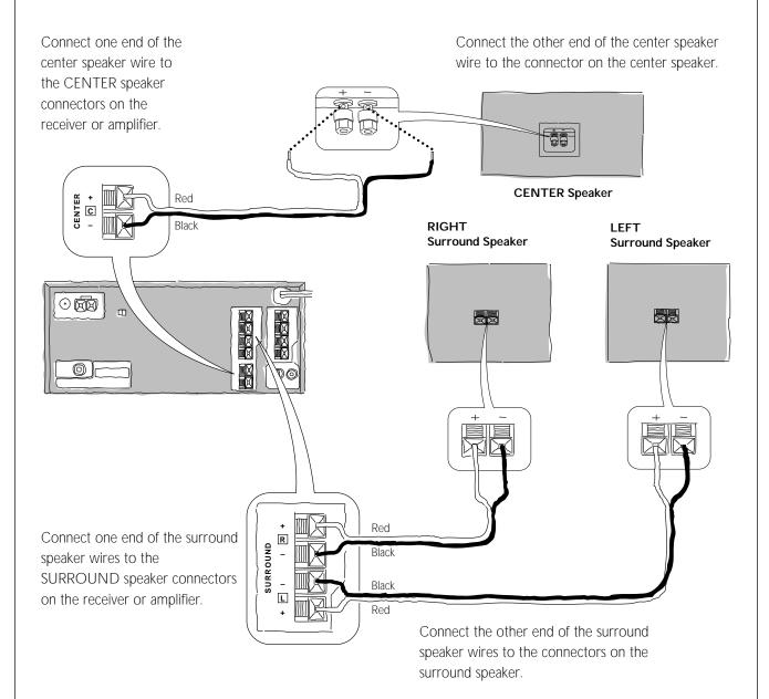
Caution: When connecting the speakers to the amplifier or receiver, be sure to always connect the positive ('+') terminals to each other, and the negative ('-') terminals to each other. Connecting the wrong terminals together could damage the amplifier or cause poor sound quality.
