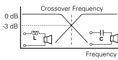
**Coil (L):** Passes low frequencies and blocks high frequencies. (Low pass)
