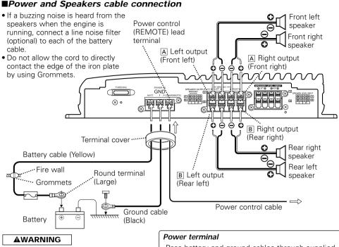
To prevent fire caused by a short in the wiring, connect a fusible link or breaker nearby the battery's positive terminal.
