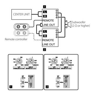
A Dual Mono Drive system is a system in which 2 monaural amplifiers are both set to bridged mode to drive one subwoofer with a high-output signal.
