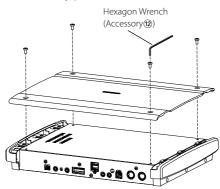
2 Use Tapping screws (Accessory⑦) to fix A/V controller Unit onto an audio board or another.
