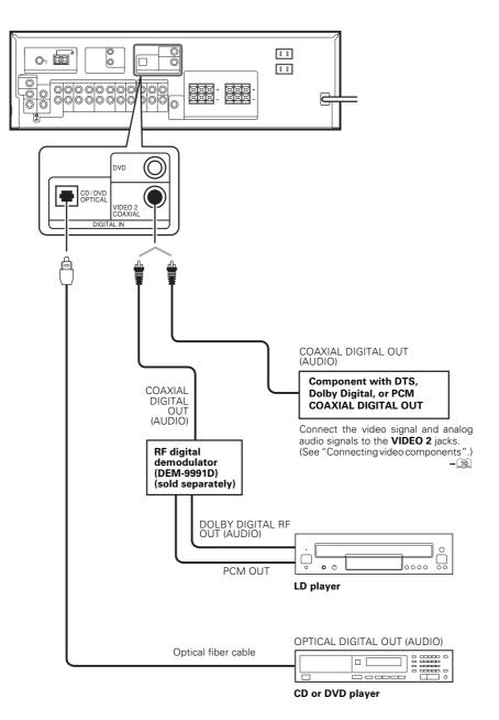
To connect an LD player with a DIGITAL RF OUT, connect the LD player to the KENWOOD RF digital demodulator (DEM-9991D). Next, connect the DIGITAL OUT jacks of the demodulator to the DIGITAL IN jacks of the receiver. Connect the video signal and analog audio signals to the VIDEO 2 jacks. (See "Connecting video components".)
