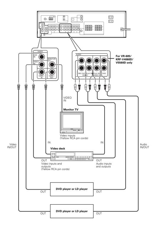
A video component with digital audio outputs should be connected to the VIDEO2 jacks.
