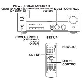
2 Turn on the power to this receiver by pressing POWER ON/ STANDBY ७ (for VR-605/615) or POWER ON/OFF and ON/ STANDBY ७ (for KRF-V5060D/V4060D/V5560D) or POWER ७ key.
