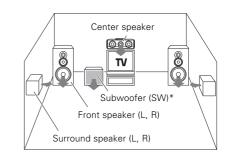
\*LFE = Low Frequency Effects. This channel delivers separate nondirectional bass singnals to the subwoofer for more dynamic deep bass sound effects.
