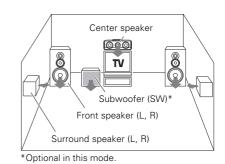
\* LFE = Low Frequency Effects. This channel delivers separate nondirectional bass signals to the subwoofer for more dynamic deep bass sound effects.
