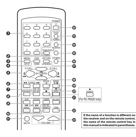
Ø Numeric keys → 23 If CD or MD is selected as the input source, these keys function as numeric keys. If tuner is selected as the input source, these keys are used to call up station presets.
