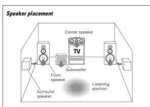
Front speakers : Place to the front left and right of the listening position. Front speakers are required for all surround modes. Center speaker : Place front and center. This speaker stabilizes the sound image and helps recreate sound motion. Required for surround playback.
