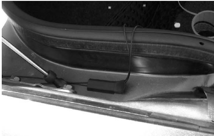
Figure 15: Cable routing along the trunk rubber molding
