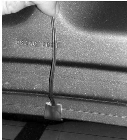
Figure 19: Routing the cables around the trunk lid rim
