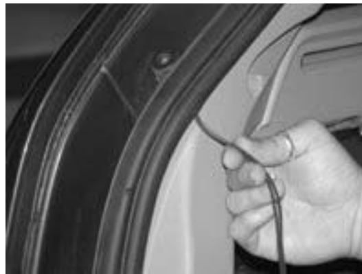
Figure 27: Hiding the cable under the rubber molding
