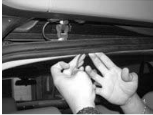
Figure 26: Cable routed through roof end and tailgate under the rubber molding
