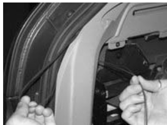
Figure 28: Going inside under the interior trim
