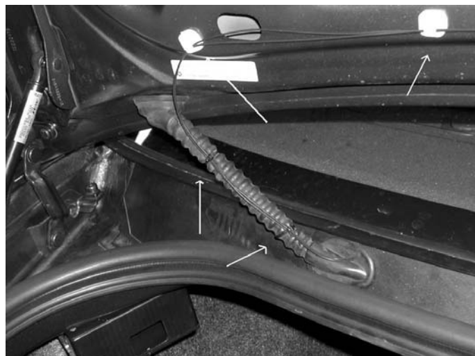
Figure 20: Attaching the cable to the cable channel
