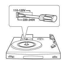
Move switch lever to match your line voltage with a small screwdriver or other pointed tool.
