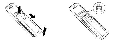
After changing remote control's RF frequency, you also must change the receiver's RF reception frequency.
