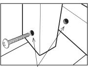
Align the predrilled holes on the leg with the metal insert on the frame, insert the bolt.
