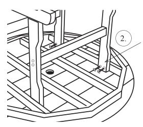
(2.) Place the leg with foot inside the frame underneath the tabletop. Align the predrilled holes, insert two 1/4 - 20 x 2 1/2" bolts then tighten them with the phillips screwdriver.
