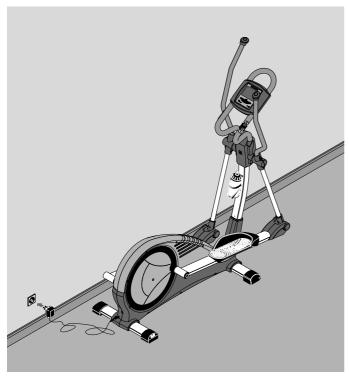
For products with power supply: **Attention!** Only use with original power unit as supplied, or with original KETTLER spare part (see spare part list). **Otherwis this may result in damage.**
