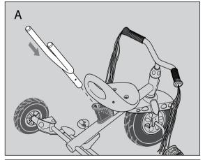
NOTE: Make sure the spring clip clicks into place when inserting the push bar shell tube.
