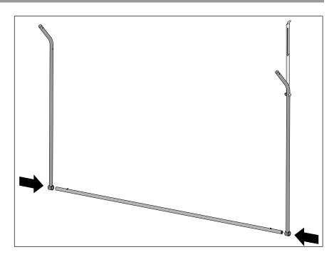
Attention: By all means, secure the table half against sliding and/or overturning for the subsequent installation steps! First, have a second person bolt the support legs attached to the table with the lateral parts.
