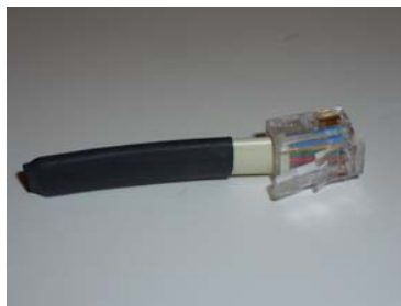
Figure 1. Modified RJ11 cable for coin unit test
