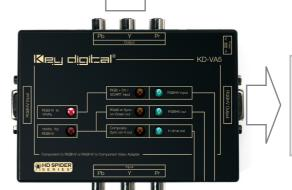
For RGBHV Video inputs, use HD-15 VGA cables and connect to the female input connector marked RGBHV Input on the unit
