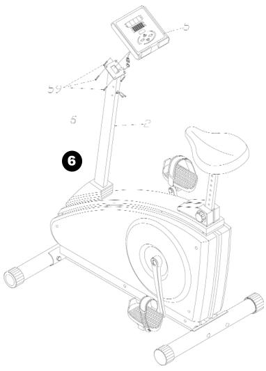
**6.** Connect the computer cable at the top of the console tube (2) to the console (5). Both computer cable connections have white ends. Feed the pulse wires from the console (5) down into the console tube (2) and out the rear hole in the handlebar area. Attach the console tube (2) to the console (5) with the screws (59) provided and already attached to back of the console (5).
