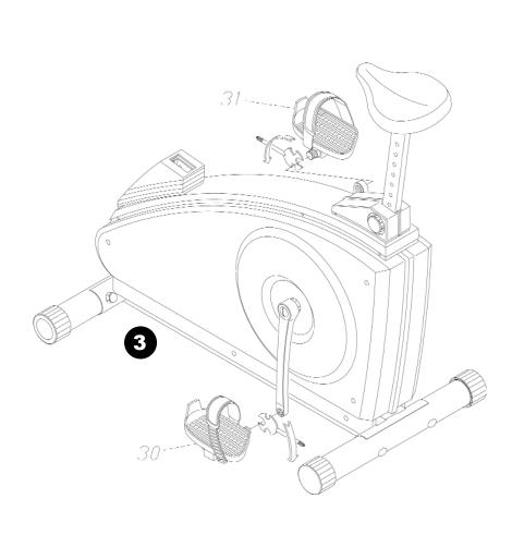
**3.** Attach pedals (30, 31). Axles of pedals are branded "L" and "R." The pedal marked "R" goes on the right hand side of the bike and the one marked "L" on the left hand side. Tighten the left pedal by turning counter-clockwise and the right pedal by turning clockwise.
