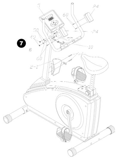
7. Attach the pulse wires in the handlebar (10) to the wires from the console (5). Connect the handlebar (10) to the console tube with the locknuts (49), flat washers (50) and screws (55) provided. Make sure not to "pinch" any of the pulse wires when connecting the handlebar to the console tube. Attach the elbow pads (24) to the handlebar (10) with screws (60). Attach bottle rack (2-1) to console tube (2).
