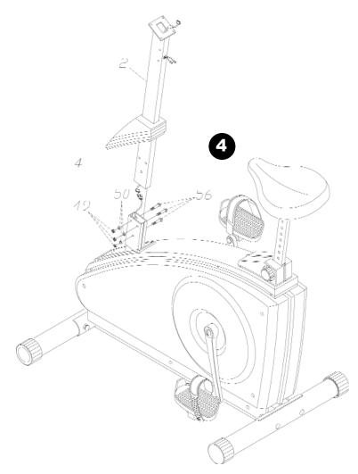
**4.** Slide the console tube (2) through the console tube collar (14, 15). Connect the computer cable in the console tube to the computer cable in the main frame. Attach the console tube (2) to the frame with the locknuts (49), flat washers (50) and screws (56) provided. Attach the console tube collar (14, 15) to the main frame (1) with screws (57).
