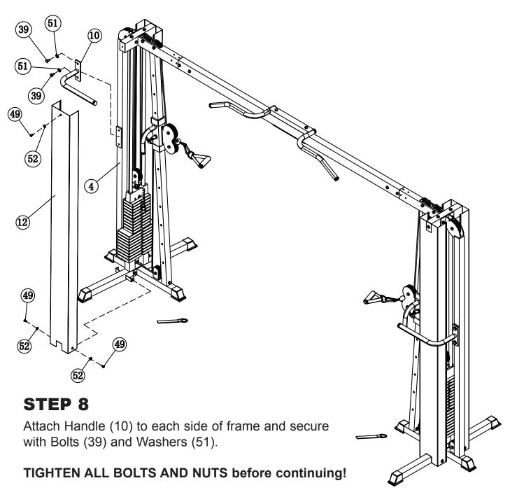
Once all bolts and nuts are tightened, then attach Weight Shrouds (12) with Allen Bolts (49) and Washers (52).
