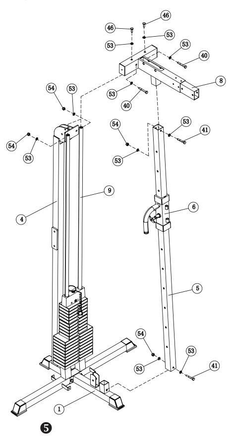
NOTE: Hand tighten bolts and nylon nuts until STEP 8.
