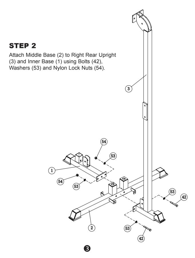
NOTE: Hand tighten bolts and nylon nuts until STEP 8.
