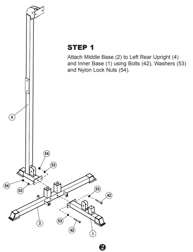
NOTE: Hand tighten bolts and nylon nuts until STEP 8.
