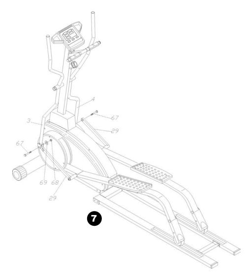
**7.** Secure the Connecting Arms (29) to the left and right handlebars (3, 4) with Screws (67), Washers (69) and Nuts (68).
