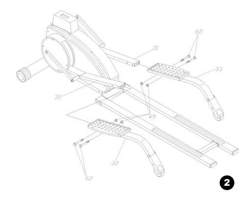
**2.** Attach both the Left and Right Rear Foot Frames (32, 33) to the Left and Right Front Foot Frames (30,31) with Screws (62) and Locknuts (49).
