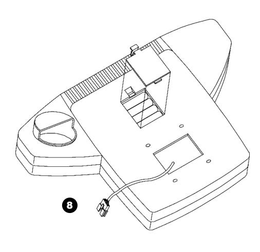
**8.** Insert the batteries provided into the back of the Monitor (5)
