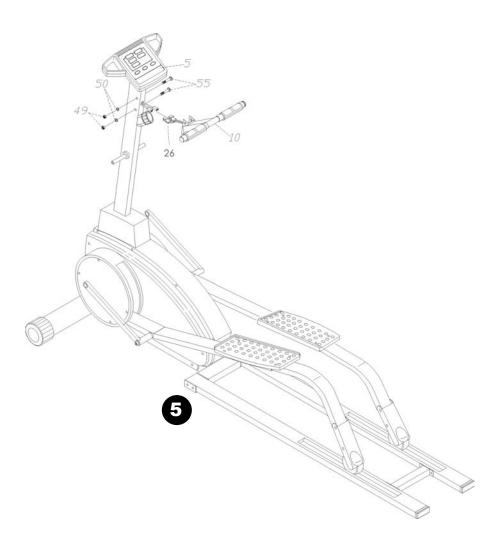
**5.** First connect the Pulse Wire (26) from the T-Shaped Handlebar (10) to the Pulse Wire from the Console. Then connect the T-Shaped Handlebar (10) to the Main Upright (2) with Screws (55), Flat Washers (50) and Locknuts (49).
