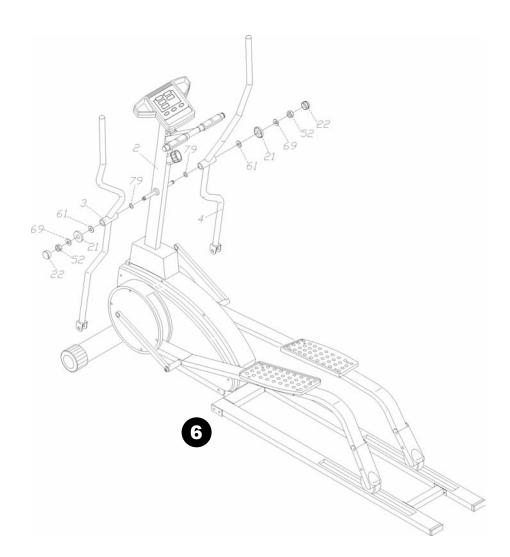
**6.** Curved Washers (79) should already be on Main Upright posts. Slide the left and right handlebars (3, 4) onto the Main Upright (2). Secure handlebars with Washers (61), Snap Caps (21), Washers (69), Nuts (52), and Bushing Caps (22).
