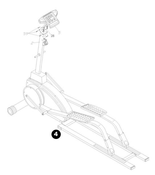
**4.** First connect the Controller Wire (28) to the Console (5). Then connect the Monitor (5) to the Main Upright (2) with the Screws (59) already supplied in the back of the Console.
