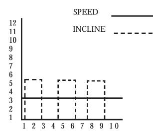
The **Weight Loss Program** is designed to vary the treadmill elevation, while maintaining a constant walking belt speed.
