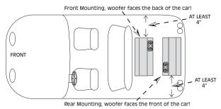
When it is more convenient to mount the enclosure along a side wall, your best option is to put it on the right side of the vehicle. (Shown below) This orientation will point the vent toward the rear of the vehicle and will produce the most low bass output. Remember to leave at least four inches of room between the enclosure and the back of the vehicle.
