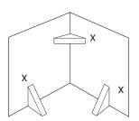
x = 3" x 3" for C15, C12 x = 2" x 2" for C10, C8 **Note:** If you prefer an ultra-smooth bass response, you should loosely fill your Comp enclosure with poly-fil (polyester fiberfill) stuffing. Ported designs will require covering the end of the port (located inside the box) with grill cloth, chicken wire, or expanded metal to prevent the poly-fil from being blown out of the port. The use of poly-fil stuffing will slightly decrease efficiency, but will deepen and extend the low frequency output.
