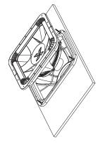
13. Using the 1/4"-20 acorn head nuts and eight bolts secure the SPAIR to the BAM. When tightening the nuts follow the pattern drawn below. This will insure a proper fit.
