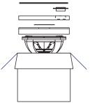
2. Once out of the carton remove the (4) four acorn head nuts and (8) eight bolts securing the SPAIR to the BAM and wood baffle assembly. *Place SPAIR in safe clean location!*
