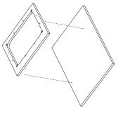
6. Once the holes are marked remove template. Using a jigsaw cutout the woofer hole and use a 3/8" drillbit for the mounting holes
