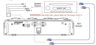
The use of twisted pair interconnects is recommended for all installations to minimize noise. When routing these cables through the automobile, try to keep them away from factory wiring harnesses and other power wiring. If you need to cross any of this wiring do so at a 90 degree angle to reduce the possibility for noise problems.
