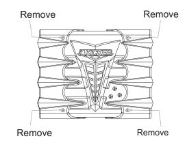
With the shroud removed, drill 4 holes using a 7/64" (2.75 mm) drill bit and use the supplied #8 screws to mount the amplifier.
