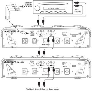
WARNING - Use either the Hi-Level or RCA Inputs. Never Both !!
