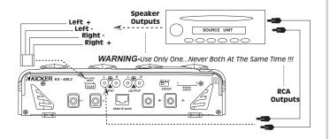
The use of twisted pair interconnects is recommended for all installations to minimize noise. When routing these cables through the automobile, try to keep them away from factory wiring harnesses and other power wiring. If you need to cross any of this wiring do so at a 90 degree angle to reduce the potential of alternator noise and electrical interference.
