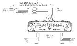
The use of twisted pair interconnects is recommended for all installations to minimize noise. When routing these cables through the automobile, try to keep them away from factory wiring harnesses and other power wiring. If you need to cross any of this wiring do so at a 90 degree angle to reduce the potential of noise problems.
