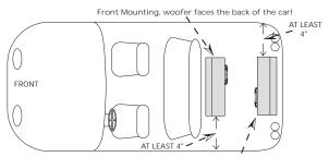
When it is more convenient to mount the enclosure along a side wall, your best option is to put it on the left side of the vehicle. (Shown below) This orientation will point the vent toward the rear of the vehicle and will produce the most low bass output. Remember to leave at least four inches of room between the enclosure and the back of the vehicle.
