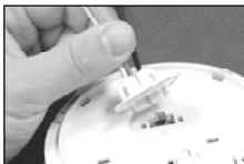
ATTACHING THE AC QUICK-CONNECT WIRE HARNESS
