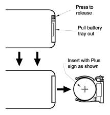
To open the battery compartment, use a fingernail to depress the release clip while pulling to the right on the battery holder.
