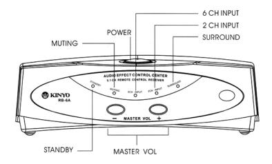
POWER: Use the button to operate power on / off
