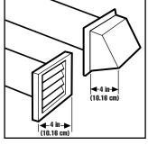
3. The exhaust vent can be routed up, down, left,
