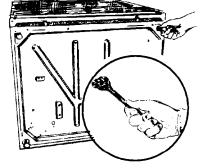
Use a 1" wrench or socket to finish turning the legs until you reach the diamond mark.
