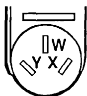
3-wire wall receptacle (10-50R)
