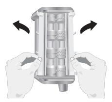
2. Remove the hopper and snap open the thin white plastic guides/levers at the bottom of the attachment for easy access to the rollers. Wash in warm, soapy water. **NOTE:** To avoid damaging the Ravioli Maker Attachment:
