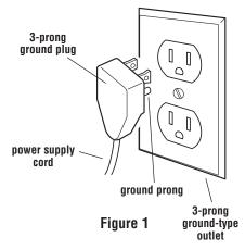
For your personal safety, this appliance must be grounded. This appliance is equipped with a power supply cord having 3-prong ground plug. To minimize possible shock hazard, the cord must be plugged into a mating 3-prong groundtype outlet, grounded in accordance with local codes and ordinances. See Figure 1. If a mating outlet is not available, it is the personal responsibility and obligation of the customer to have a properly grounded 3-prong outlet installed by a qualified electrician.
