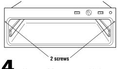
■ Use two (2) screws provided to secure the warming oven frame to the cabinet.
