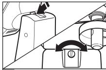
Lift motor head. Turn screw slightly counterclockwise (left) to raise flat beater or clockwise (right) to lower flat beater. Make adjustment with flat beater, so it just clears surface of bowl. If you over adjust the screw, the bowl lock lever may not lock into place.
