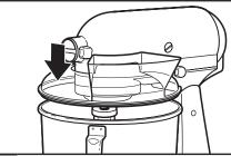
2 From the front of the Stand Mixer, slide the pouring shield over the bowl until the shield is centered. The bottom rim of the shield should fit within the bowl.
