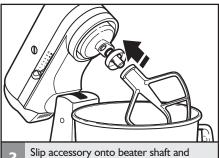
Slip accessory onto beater shaft and press upward as far as possible. Then, turn accessory to the right, hooking accessory over the pin on the shaft.
