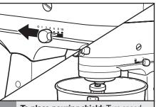
To place pouring shield: Turn speed control to "O". Unplug Stand Mixer. Attach your chosen accessory, see "Attaching/removing the flat beater, wire whip, or dough hook" section.
