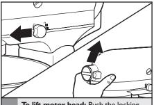
To lift motor head: Push the locking lever to the UNLOCK position and lift the head. Once lifted, the lever will automatically go back in LOCK position to keep the head lifted.
