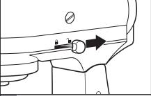
To put down motor head: Push the locking lever to UNLOCK and gently bring the head down. The locking lever will automatically go back in LOCK position when the head is down. Before mixing, test lock by attempting to raise motor head.
