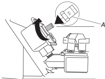
A. Number 46 Natural gas bake burner orifice hood
