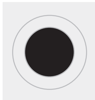
Fig. 2 Heating with inner (small) element only
