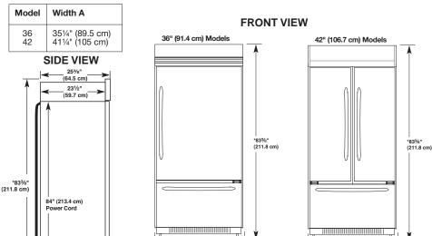
When leveling legs are fully extended to 11/4" (3.2 cm) below rollers, add 11/8" (2.9 cm) to the height dimensions.
