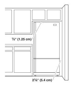
To ensure proper ventilation for your refrigerator, allow for 1/2" (1.25 cm) space on each side, at the top and behind the refrigerator. When installing your refrigerator next to a fixed wall, leave 2 1/8" (5.4 cm) minimum on the hinge side to allow for the door to swing open. If your refrigerator has an ice maker, allow extra space at the back for the water line connections.
