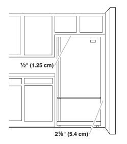
To ensure proper ventilation for your refrigerator, allow for 1/2" (1.25 cm) space on each side, at the top and behind the refrigerator. When installing your refrigerator next to a fixed wall, leave 2 1/8" (5.4 cm) minimum on the hinge side to allow for the door to swing open. If your refrigerator has an ice maker, allow extra space at the back for the water line connections.
