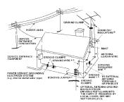
NOTE TO CATV SYSTEM INSTALLER: This reminder is provided to call the CATV system installeris attention to Article 820-40 of the National Electrical Code that provides guidelines for proper grounding and, in particular, specifies that the ground cable ground shall be connected to the grounding system of the building, as close to the point of cable entry as practical.
