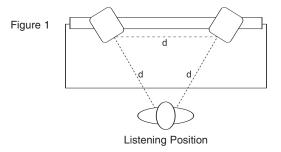
**Mid-Field Configuration:** This configuration is essentially the same as the Close-Field setup (see Figure 2). The Mid-Field configuration is normally used with larger monitors or when the monitors are too large or heavy for the meter bridge, as is likely the case with the Exposé E8B. This set-up has the potential for a larger sweet spot and better spatial imaging. Ensure that the height of the woofer is above the height of the console's meter bridge.
