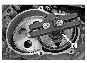
Screw the extractor (special tool item no. 590.29.021.044) onto the clutch hub [6] with the M5x50 screws, hold the extractor and remove the centrifugal clutch from the crankshaft by screwing in the extractor screw. Completely remove the centrifugal clutch, bearings and spacing washers from the crankshaft.
