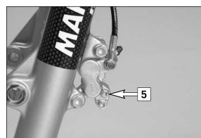
Mount the left brake shoe and fix with screw. Mount the right brake shoe and tighten the screw to 4 Nm. Mount the lock washer. Align brake shoes, mount front wheel (see chapter: Mounting the front wheel).
