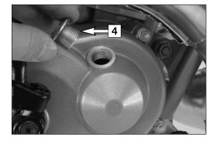
Remove stopper **[4]** and fill in 0.15 liters of automatic gear oil (Motorex ATF Super). Mount the stopper and check the engine for tightness.
