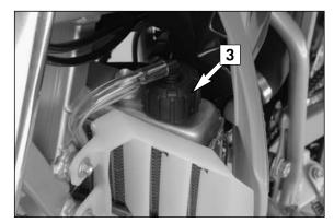
A mixture of 50 % antifreeze and 50 % distilled water is used as the cooling liquid. How-ever, the antifreeze protection must be at least  $-25^{\circ}$  C ( $-13^{\circ}$  F). This mixture offers antifreeze protection but also good corrosion protection and should therefore not be replaced by pure water.
