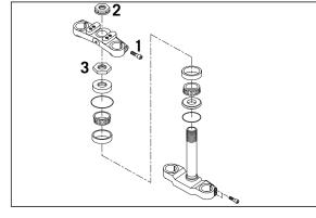
At least once a year, the steering head bearings should be smeared with waterproof grease (Motorex Long Term 2000).
