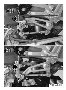
The position of the shift lever can be greatly varied, depending on the length of the shift rod and the drill holes selected. As seen from the footrest, there is either a high position of the shift lever ① or a low position of the shift lever ③.
