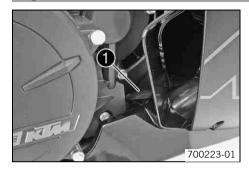
The engine number • is stamped on the right side of the engine.
