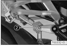
Turn the eccentric shaft 2 to the desired position using the tool from the tool set.
