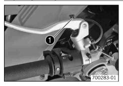
Adjust the basic setting of the clutch lever to your hand size by turning adjusting screw •.
