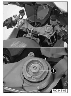
Turn the adjusting spindles ① clockwise until they stop.
