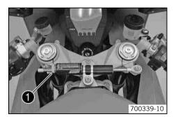
Turn the adjusting screw • anticlockwise towards "-" as far as the last perceptible click.  Adjust the steering damper according to your riding style and the road conditions by turning the adjust screw clockwise towards "+".
