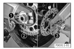
Remove nut 1. Remove chain adjuster 2. Withdraw the wheel spindle 3.
