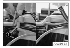
By removing or inserting the spacing sleeves  $\mathbf{0}$ , you can set the handlebar height at two different positions.
