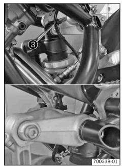
When you screw in the rear left fixing screw, the plug-in cable binder 3 is pushed out of the thread. To reposition the cable of the lambda probe, fix the plug-in cable binder in the remaining free drill hole.
