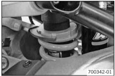
Turn the adjusting ring anticlockwise with the toolset wrench until the spring is completely relaxed.
