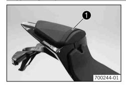
The supporting strap • is provided for the passenger to hold on to.
