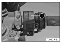
The emergency OFF switch  $\bullet$  is fitted on the right side of the handlebar.
