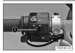
The flasher switch **1** is fitted on the left side of the handlebar.
