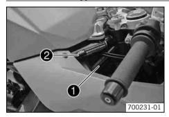
The chassis number **1** is stamped on the frame behind the steering head on the right. The type label **2** is on the frame above the chassis number.
