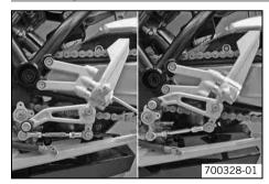
The adjustable footrest system enables an individual setting of the footrest height and an individual adjustment of the operating elements.
