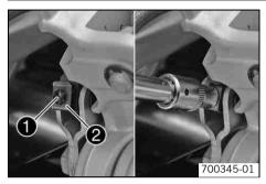
– Use the tool to press in the anti-rotation lock  $oldsymbol{0}$ , then turn the piston rod  $oldsymbol{0}$ .
