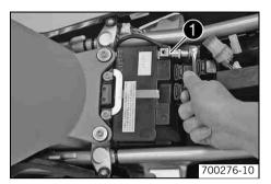
Disconnect the negative (minus) cable ● of the battery.
