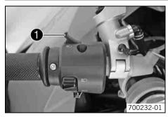
The headlight flasher switch • is fitted on the left side of the handlebar.
