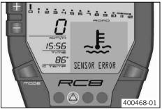
**SENSOR ERROR** appears on the info display if the coolant temperature between the coolant temperature sensors of the front and rear cylinders differs by more than the specified value.
