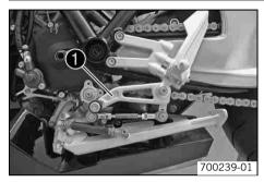
The shift lever **1** is mounted on the left of the engine.
