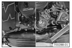
Fit and tighten the oil drain plug with the magnet, O-rings and oil screen.
