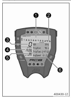
The tachometer ① displays the engine speed in revolutions per minute (RPM). The red marking ② marks the over-rev (excessive speed) range of the engine. The speed ③ is displayed in kilometers per hour **km/h** or in miles per hour **Mph**. The time appears in segment ④.
