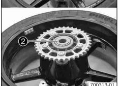
Remove bushing 1 and bushing 2. Clean and grease the roll surfaces of the bushing and the shaft seal rings.
