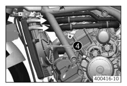
Cooling takes place by means of the air stream and a radiator fan **4**, which is controlled by a thermoswitch.
