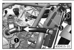
The water pump with a 3D water pump wheel **1** in the engine ensures forced circulation of the coolant. The heat exchanger enables faster warming of the engine oil at the start of a journey and better heat dissipation for the engine oil during the journey.
