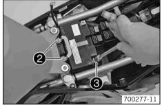
Mount and tighten screws ②.
