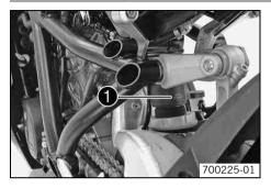
The shock absorber part number lacktriangle is stamped on the upper part of the shock absorber above the adjusting ring towards the rear.
