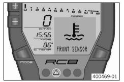
**FRONT SENSOR** appears on the info display if the coolant temperature sensor of the front cyclinder is defective.
