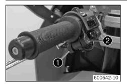
The **Mode** button  $\bullet$  is fitted on the handlebar, front left. The **Lap** button  $\bullet$  is fitted on the handlebar, rear left.
