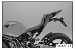
Tighten the screw on the left and right sides of the vehicle.
