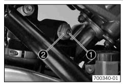
The shock absorber can coordinate the compression damping separately in the low **1** and high **2** speed range (Dual Compression Control).
