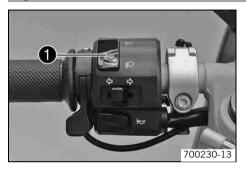
The light switch **1** is fitted on the left side of the handlebar.
