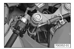
Loosen the clamp screws of the lower and upper triple clamps and of the handlebar stub.
