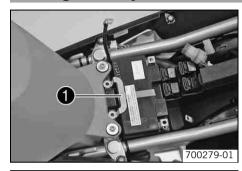
Position the battery in the battery rack.
