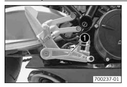
The footbrake pedal **1** is in front of the right footrest. The footbrake pedal operates the rear brake.
