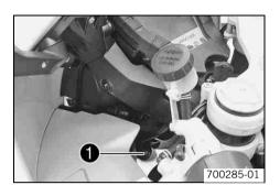
Adjust the beam distance of the headlight by turning screw ①.
