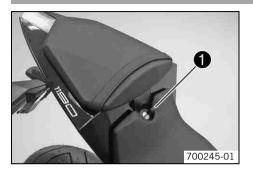
The seat lock • is behind the seat. It can be locked with the ignition key.
