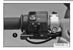
The horn button • is fitted on the left side of the handlebar.
