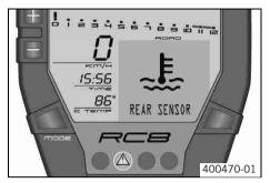
**REAR SENSOR** appears on the info display if the coolant temperature sensor of the rear cyclinder is defective.
