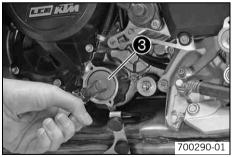
Pull the oil filter element 3 out of the oil filter case.
