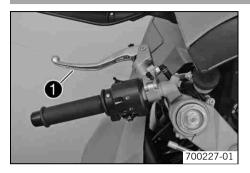
The clutch lever **①** is fitted on the left side of the handlebar. The clutch is hydraulic and self-adjusting.
