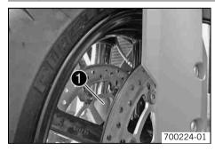
The fork part number **1** is stamped on the inner side of the fork stub.
