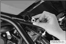
Fit the screw and washer on the left and right sides of the vehicle, and tighten.
