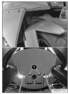
Remove screws 1. Remove cover.
