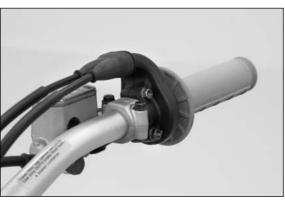
Mount the front wheel fender and tighten the screws to 10 Nm. Mount the hand brake cylinder and tighten the screws to 10 Nm. Mount the staring number plate.
