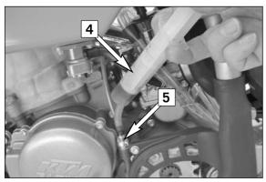
Fill the bleeder syringe [4] with a suitable fluid (see Technical Specifications - Engine). Remove the bleeder screw from the slave cylinder [5] and mount the bleeder syringe.
