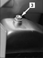
Remove screw [2] at the cylinder head. Reinstall it as soon as the cooling liquid emerges free of air bubbles (only for 125/200 engines).
