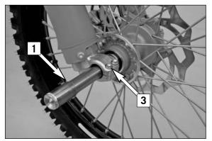
To install the front wheel, lift it into the fork, position and mount the axle shaft [1]. Mount the collar nut [2], tighten the clamping screws [3] on the right fork leg axle passage to prevent the axle shaft from turning and tighten the collar nut to 40 Nm (30ft.lb).
