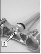
Remove the collar screw from the lower triple clamp and pull out the steering stem. Thoroughly clean all parts. Turn the steering stem  $180^{\circ}$  and insert it in the triple clamp. Apply Loctite 243 to the thread of the collar screw [2] and turn all the way in.
